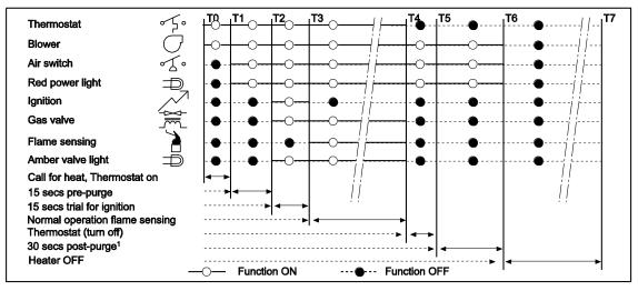
Note: When the tube heater is operated by a thermostat interrupting the line voltage (120V) to the heater then the post purge function is disabled.
