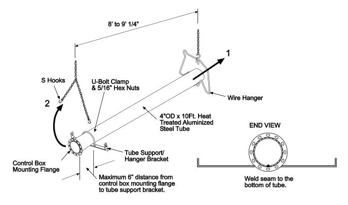
5. Suspend the chain to attach the wire hanger and the tube support bracket. Insert the tube into the wire hanger and then raise the tube support bracket end up to the suspension chain, use "S" hooks to attach the wire hanger and tube support bracket to the chain.
